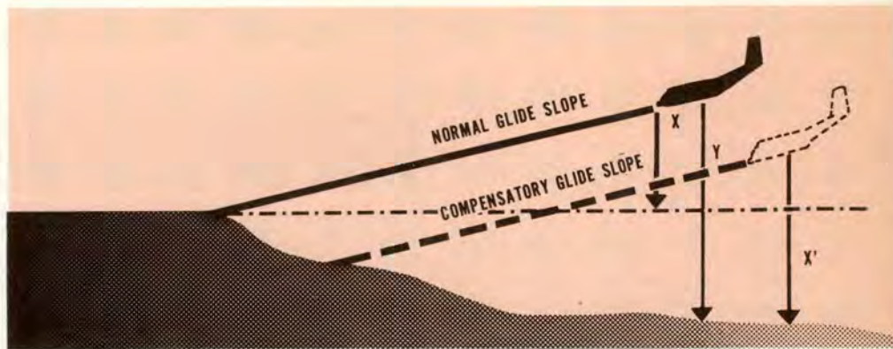
The effect of terrain downslope in the runway approach on aircraft glide slope. With a terrain downslope, the pilot will believe the aircraft to be on low, flat approach, and there is a tendency to land short of the runway.
